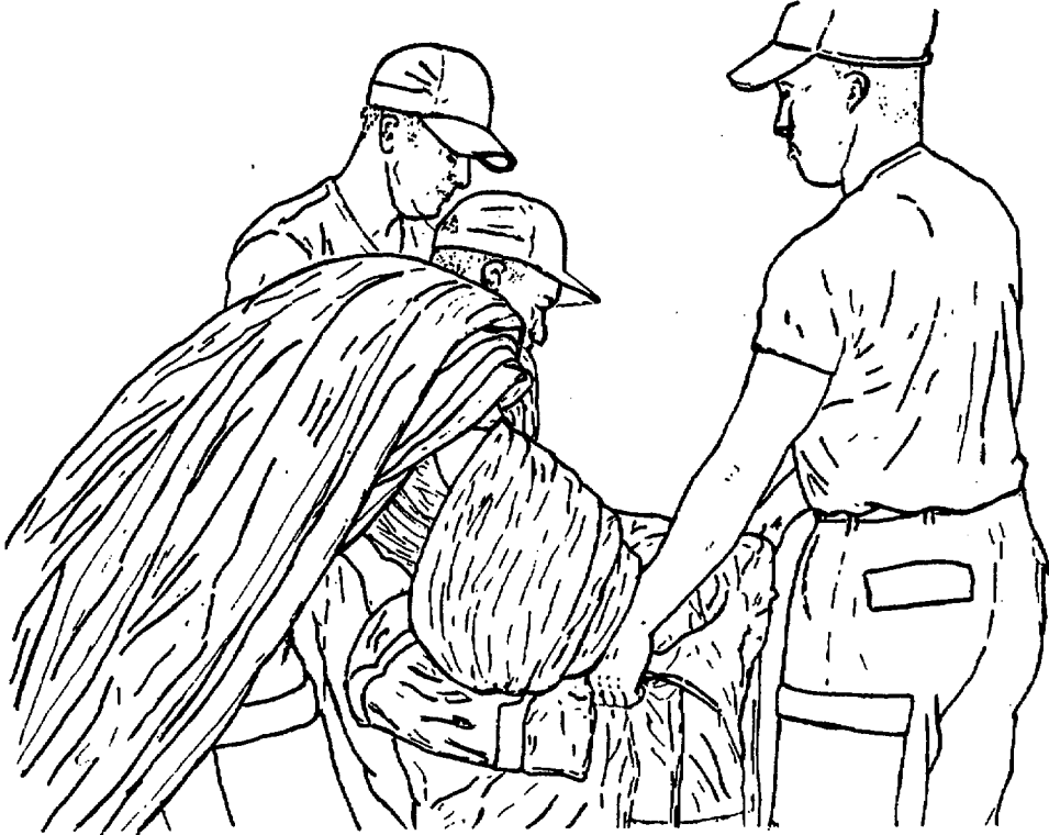
Figure 2-30. Stowing the Canopy in Deployment Bag.
